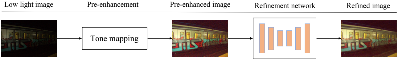
Fig. 2. Diagram of the proposed two-stage framework for low light image enhancement. Given a low light image, in the first stage, we employ the tone mapping method proposed in [1] to pre-enhance the image. In the second stage, we use a refinement network for further improvement of image quality.
