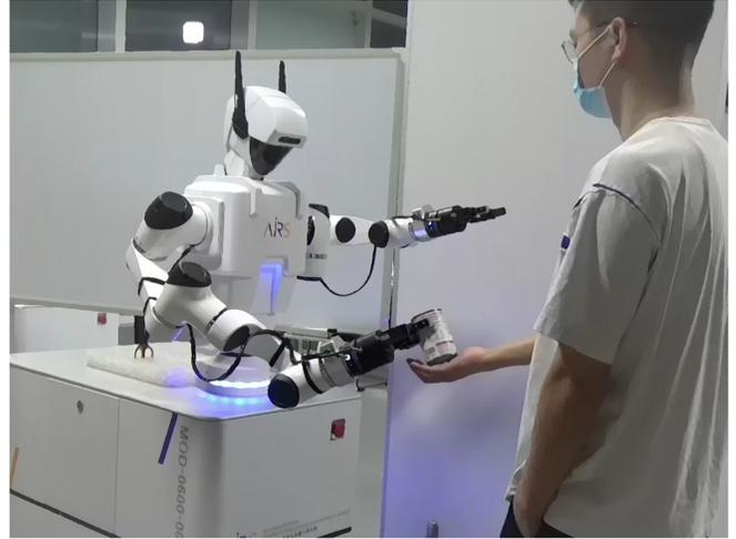
Fig. 1: Robots transport object that human hands can grasp comfortably. Our system first predicts a suitable grasp for the human hand, then based on the human hand tracking and reconstruction, it delivers the object to the human and can adapt to the scene of the human hand moving.
