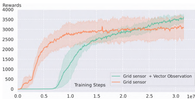
Fig. 13. Comparison of two different observations. The pink line indicates the situation where the team of catcher robots uses grid sensors as observations. The green line indicates the situation in which the team of catcher robots uses grid sensors together with the location of the runner robots as observations. We can see that when the location information is given to the catcher robot team, they are able to get more rewards in the environment, indicating that the catcher robots can suspend the runner robots more.
