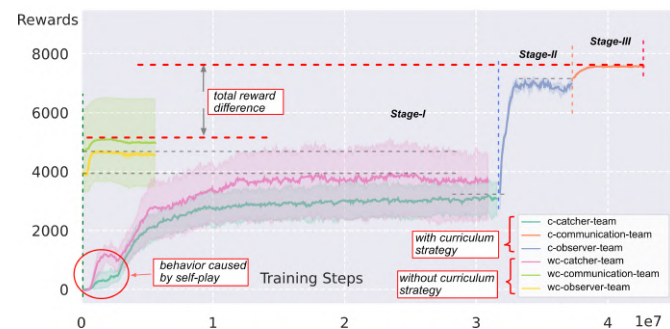
Fig. 10. Illustration of the learning curves of our system. Two groups of curves are compared in this figure. One group, which consists of pink, yellow, and green curves, is trained without the curriculum strategy. The other group, which consists of green, blue, and red curves, is trained with the curriculum strategy. A total reward difference can be found between the two groups.
