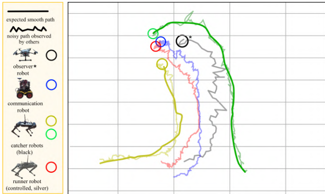
Fig. 21. Paths generated by different robots in the outdoor environment. Although the robots are affected by noises and do not generate the expected smooth paths, our system can still finish the task. * The noisy path of the quadcopter is extracted post-experiment from video, and the noisy paths of other robots are recorded by the UWB device during the experiment.
