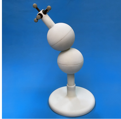
Fig. 1: A dexterous joint by driving-integrated spherical gears and have recently attracted increasing interest from robotics communities [6, 7].
